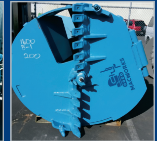
Gated Clay Drilling Bucket
