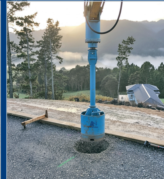
Gated Clay Drilling Bucket
