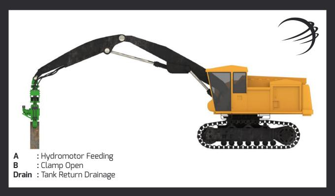
Our excavator mounted vibratory hammers are attached easily to excavator pump system and can be operated in a very short time. A line is a feeding line for hydromotor and B line is for clamp open action. Drain line is a connection from hydromotor oil leakage to excavator tank.
